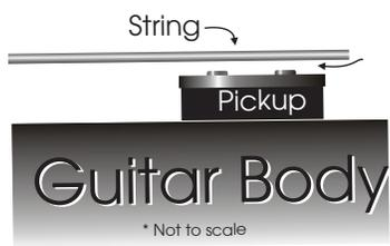
Starting distance between string and pickup blades should be 4/32" on the bass side and 3/32" on the treble side when the strings are fretted at the higher frets. Raise or lower from here to suit your playing style and your desired tone.
