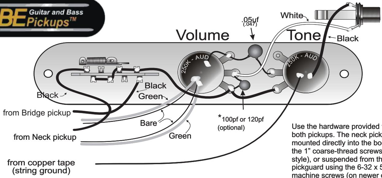
Red & White wires are soldered together and insulated with heat shrink. For typical Tele-style operation do not disturb this connection.
