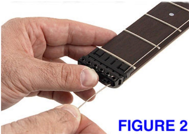
Pull non ball end of string through the nut and through the appropriate hole in the adapter. (FIGURE 2)
