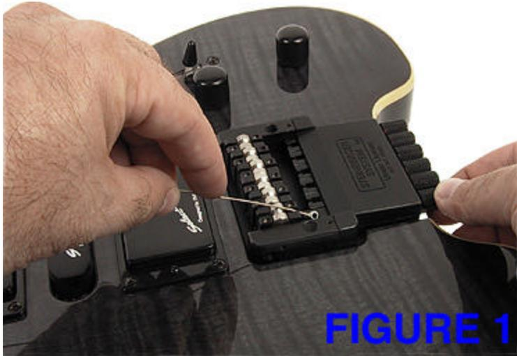
Loosen the tuning machine and insert ball end. Close machine just enough to where ball end will not come out of machine. (FIGURE 1).
