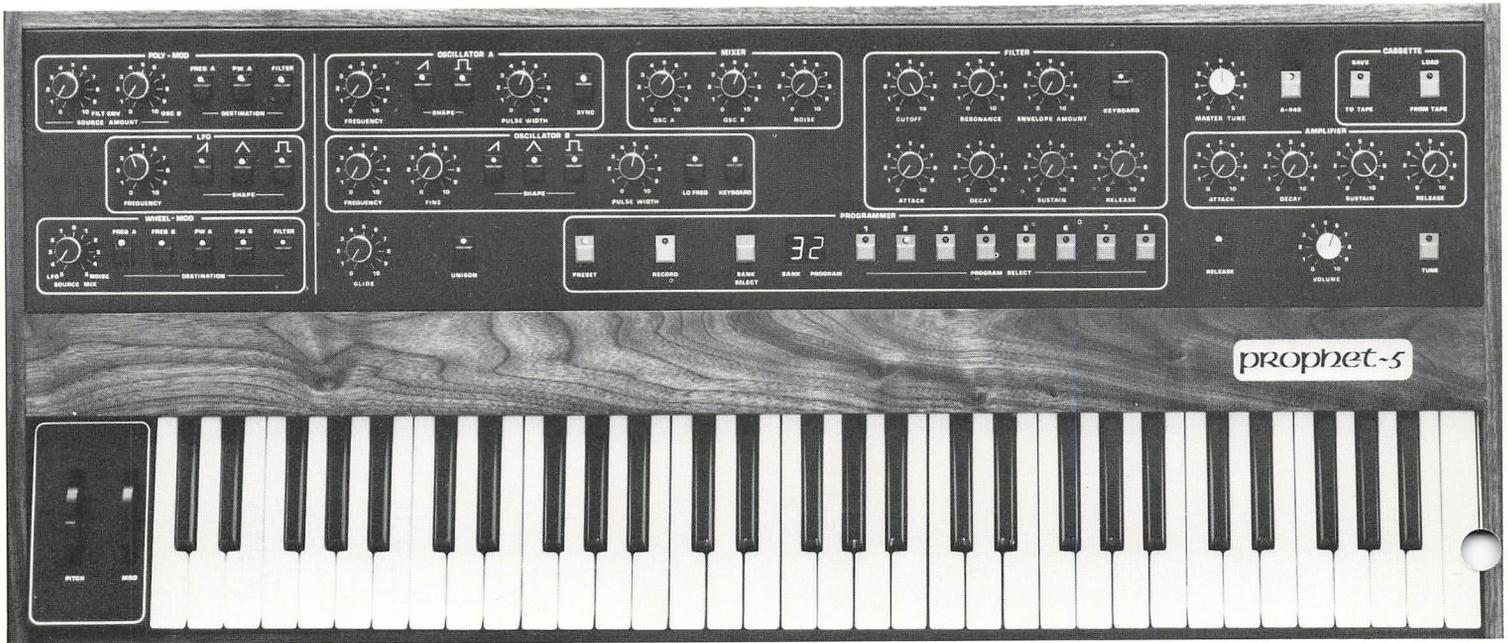
The **PROPHET 5** from Sequential Circuits is a completely programmable polyphonic synthesizer, the world's first in fact. The **PROPHET** has 5 complete voices with two voltage controlled oscillators, a noise source, a voltage controlled lowpass filter and two 4 stage envelope generators per voice. The voices can be controlled by either the front panel knobs and switches or by one of the programs in storage.
