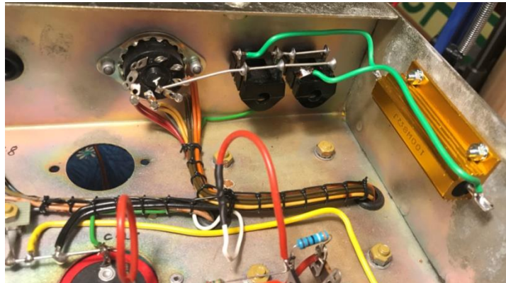
Final design: output topology with 8\Omega/100W power resistor
