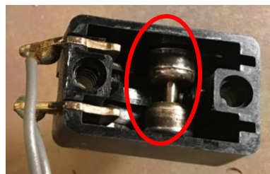
Open standby switch corroded
