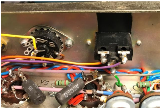
Previous design without EMC protection
