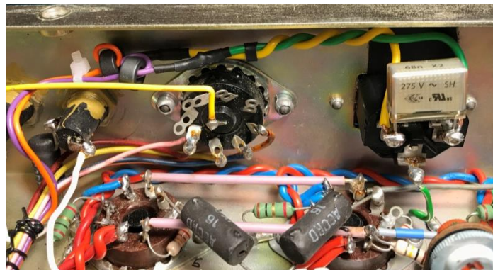
Final design with X2 capacitor and 2 ferrite rings
