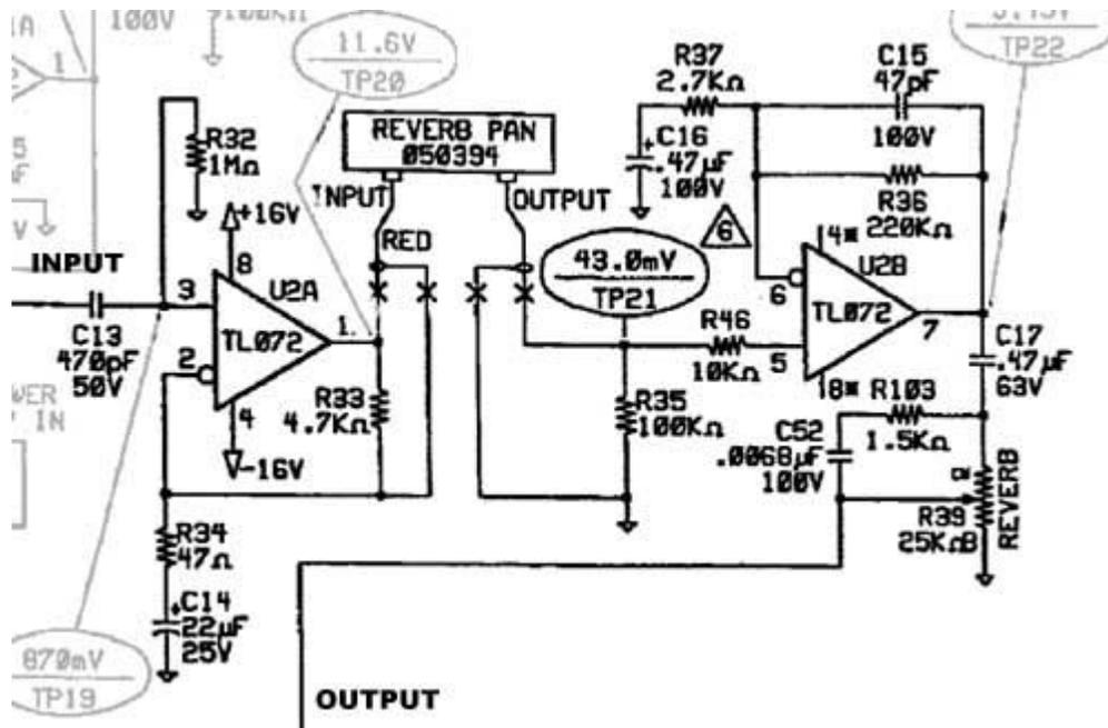
It's well known that the Hot Rod uses TL072 opamps, but how is the reverb implemented? The reverb driver opamp is a "current driver." This simulates the old transformer coupled tube circuits much better than other voltage driven opamp circuits.
