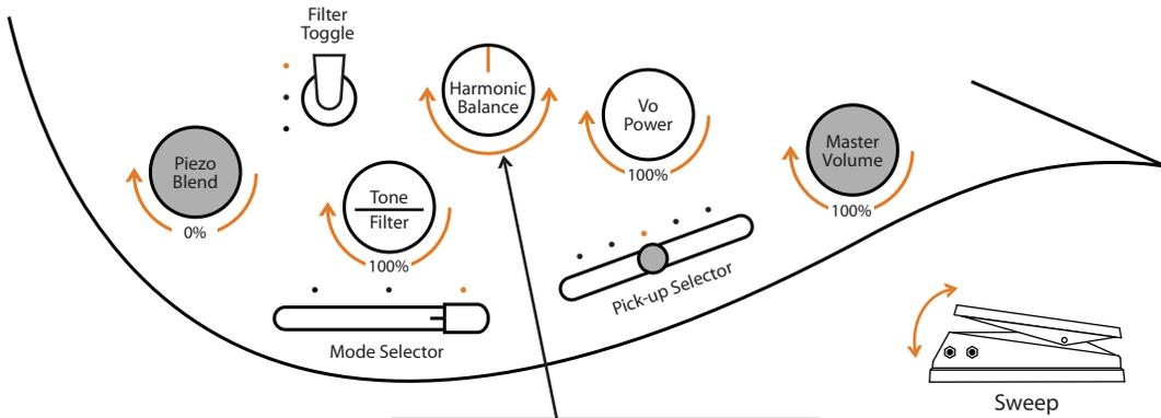
Sweep the Harmonic Balance knob to create Harmonic Blends while in the Moog Filter or Articulated Moog Filters modes. Return to center for maximum sustain.
