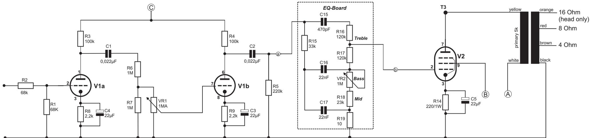
The EQ-board is connected with 3 wires (white, red and black) to points a and b on the main PCB.
