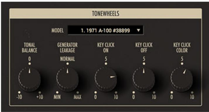
This section of the panel adjusts the tonewheels, the actual sound generators of the organ. The hardware Hammond organ uses 91 spinning tonewheels to generate all of the needed pitches in the instrument. The tones are mixed together in a matrix based on the drawbar positions and the notes played. Here you can control the tonewheels further.
