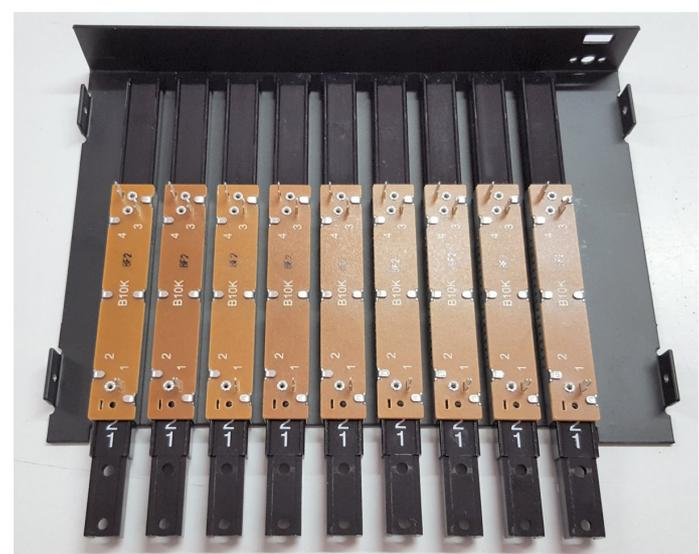
**STEP 9:** Fix the PCB assembly to the drawbars and solder the DIL terminals. Slide the boards slightly angled so the MicroUSB connector can easily pass through the hole in the metal panel.
