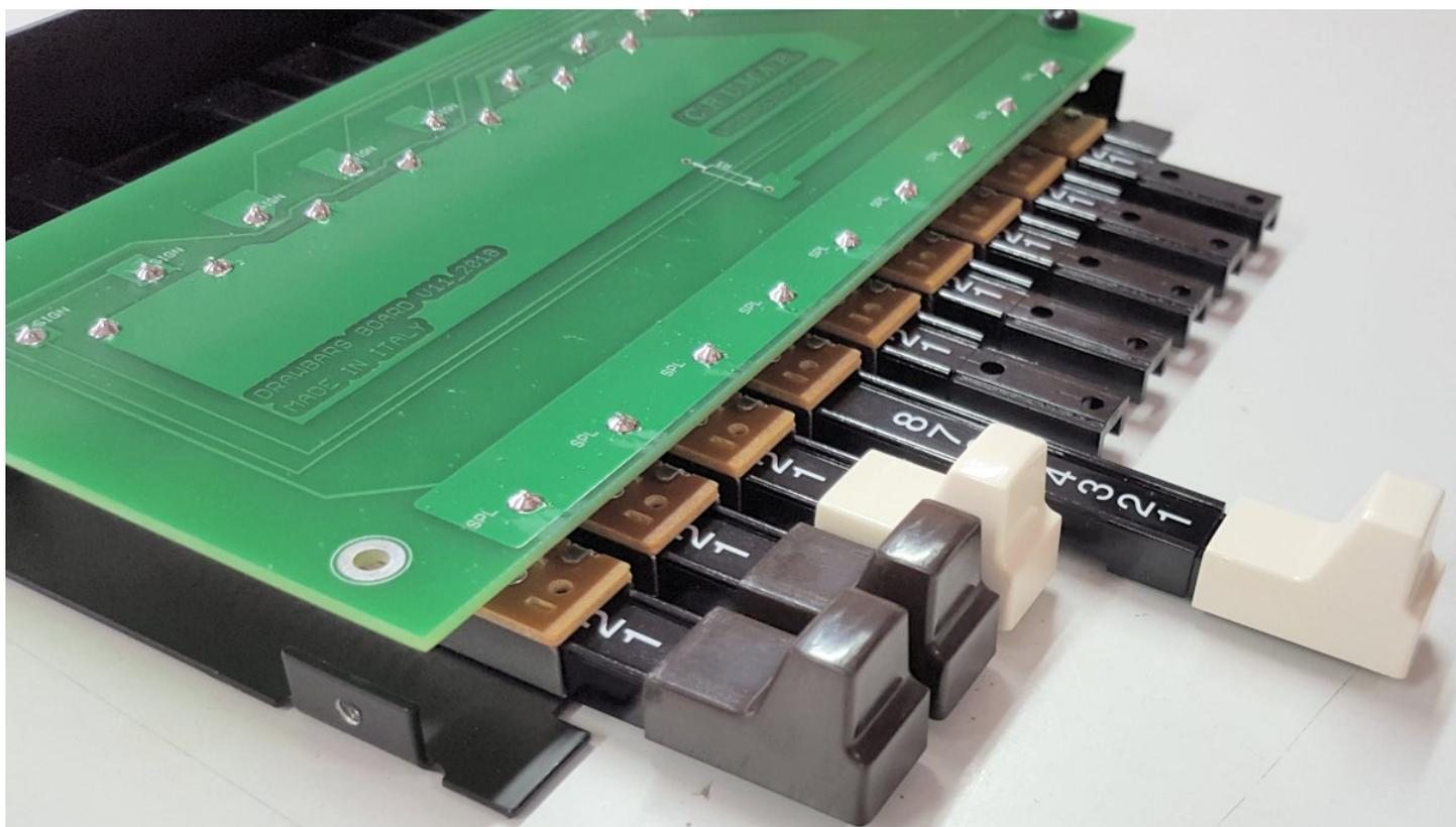
Once done, turn the whole assembly upside down and fix them using the 9 M3X6 screws.
