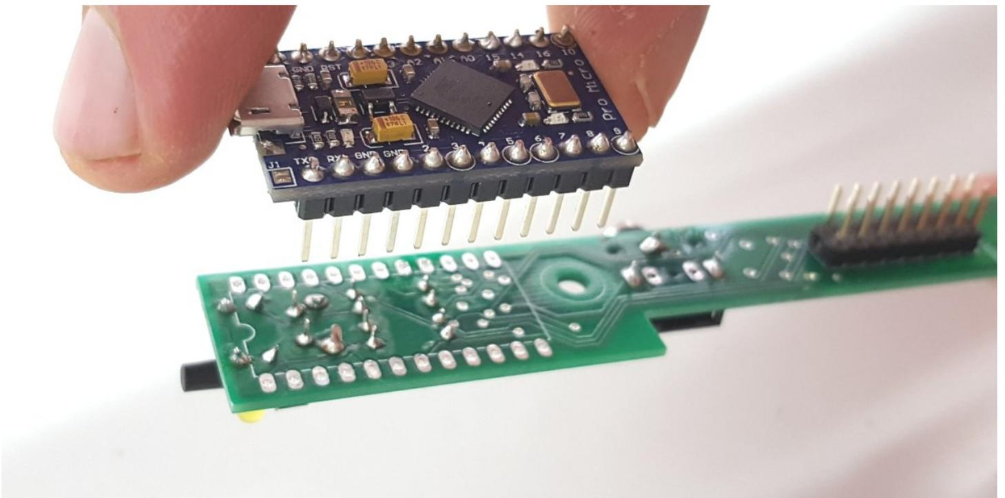
**STEP 6:** Once soldered the CPU board, the final assembly should look like the picture below.
