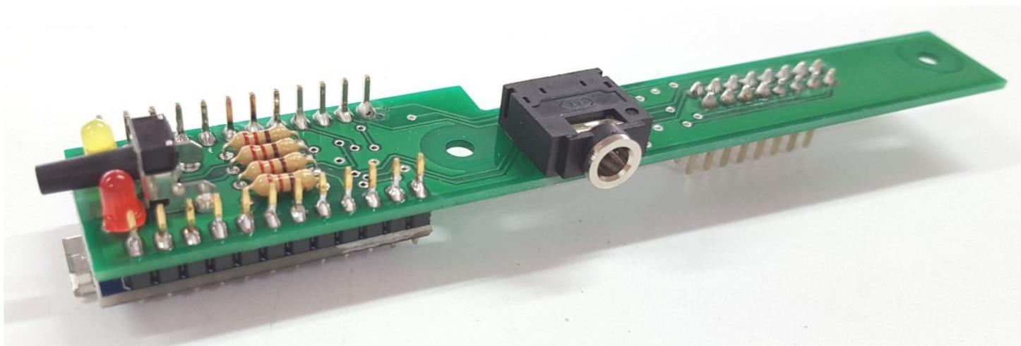
Now take your cutters and cut the exceeding terminal strip leads on the JACK side, as shown below. Optionally, you can also cut the exceeding leads on the other side.
