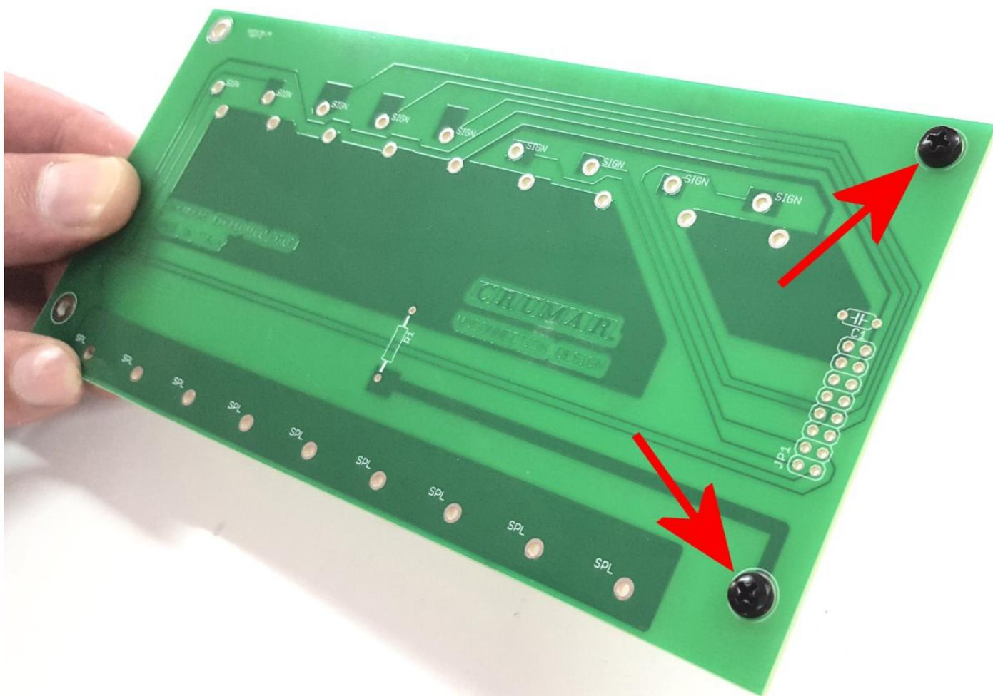
Then, insert the spacers on the other side, add the main board and fix the bolts using your fingers to hold the bolts and a screwdriver to tighten the screws.
