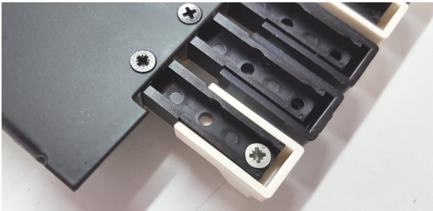
**STEP 12:** Put the metal top cover. In order to have the jack connector easily pass through the hole in the metal panel, start from an angle from the connector's side.
