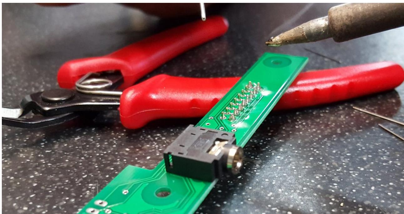
**STEP 4:** Take the CPU board and solder the SIL terminals to the tiny board. This board contains active SMT electronics and is subject to ESD and overheat, make sure that your soldering iron doesn't exceed 350 °C (~660°F) and don't keep the soldering pin on the terminals for too long. The SIL strip must face the bottom of the board, thus the pins will be soldered on the top side, as shown in the picture below.
