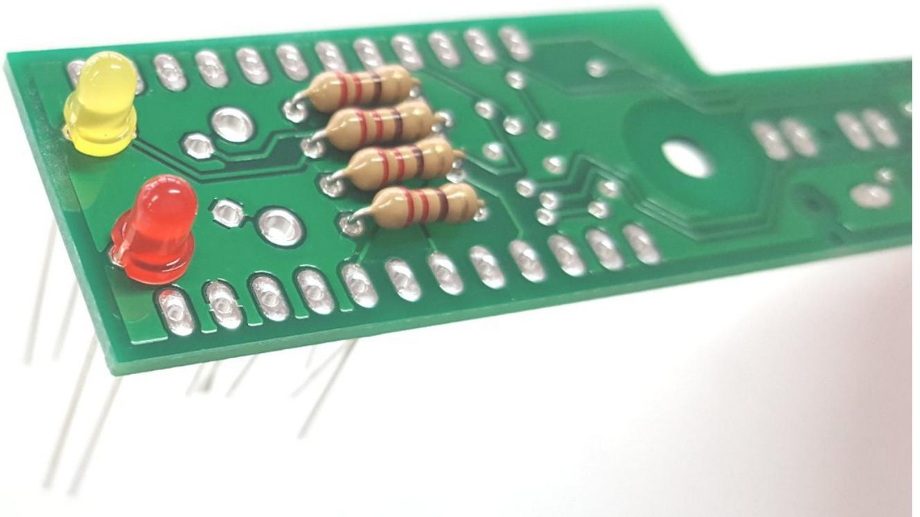
Proceed with the soldering of these first components and cut the exceeding leads.
